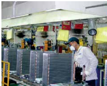
Outdoor units production
